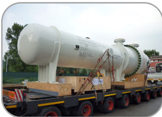
(up) 1 of the 4 EMbaffle® units for Overhead Condensing (down) 1 of the 2 EMbaffle® units for the Gas Compression after-cooling
